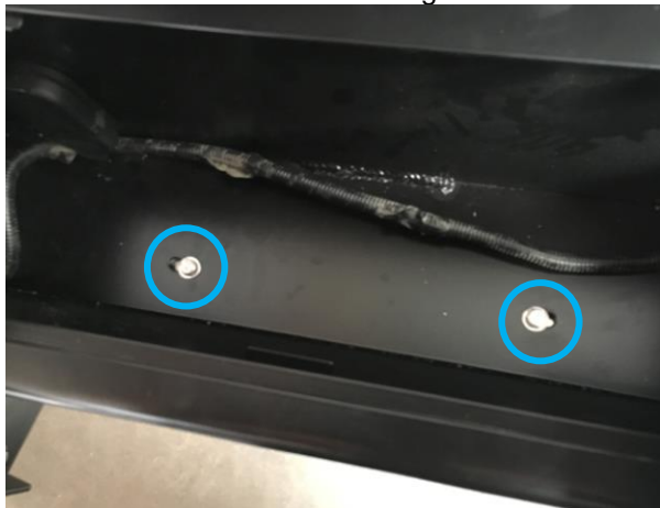
Figure 6: Lower "L" Brackets Tightened onto Bumper
