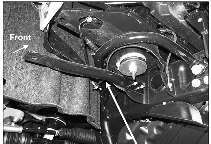
(Fig 4) Remove outer bumper support brackets
